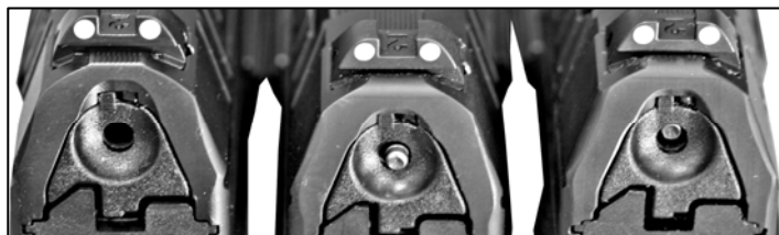
2.4 Fig. 2, from left to right: de-cocked, cocked, cocked (P99 QA only)
