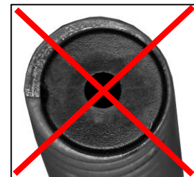
4.1 Fig. 8 Improper alignment spring not centered
