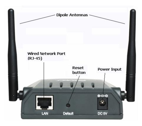
The EZ Connect $^{\text{TM}}$  g 54 Mbps Wireless Ethernet Bridge has three types of LED indicators. Please check the following picture – the front view of the Bridge and the table below, which displays the current state the specific LED signifies.
