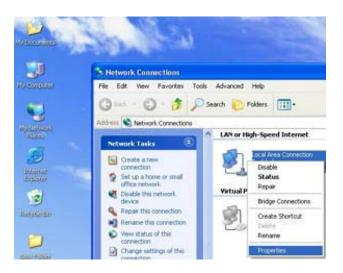
3) Click "Internet Protocol TCP/IP" and click "Properties". Select the "Use the following IP Address" option and insert 192.168.2.x (where x is 2 ~ 24, 26 ~ 254) for the IP address. If requested to enter a gateway and DNS, you can type in 192.168.2.1.
