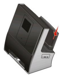
**Note:** Do not force paper into the printer. The paper should be flat against the paper support, and the edges should be flush against both paper guides.
