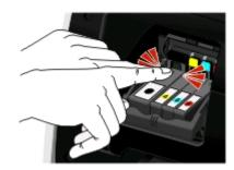
**Note:** Install the new ink cartridges immediately after removing the protective cap to avoid exposing the ink to air.
