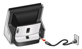
**3** After a minute, reconnect the power cord into the power supply.
