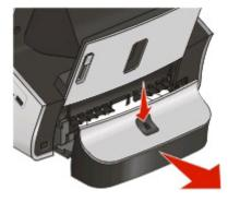
CAUTION—POTENTIAL INJURY: The area behind the duplex cover has protruding ribs as part of the paper path. To avoid injury, use caution when accessing this area for clearing a paper jam.
