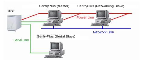
If there is a communication cable between the computer and a UPS, this computer called Master. The Master can monitor and control the connected UPS directly, as it also transmits the UPS information to the Slave(s).
