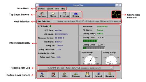
**Host Selection**: Press the combo box to select hosts that runs SentryPlus Service in the LAN. Users can monitor or control (need password) remote UPS.
