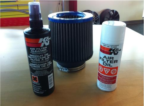
Over a sink, spray the cleaner on the OUTSIDE of the filter.
