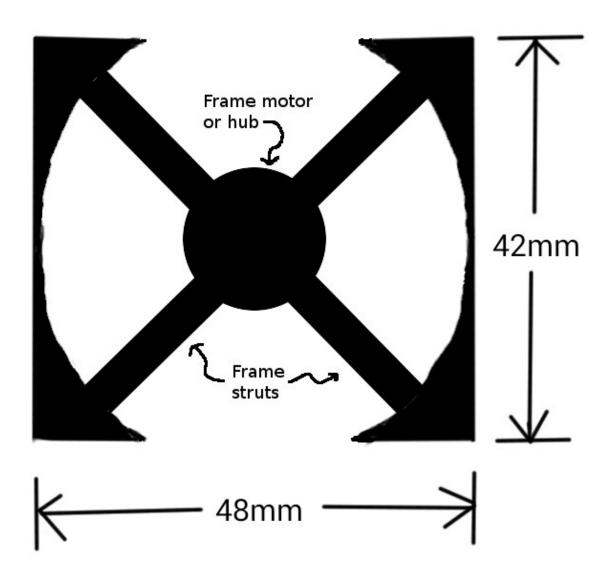
Fig. 2 Example drawing of fan with disappearing top and bottom frame segments.
