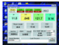
Windows® Software included to monitor readings on PC, display KWH, KWH/month, cost and print reports
