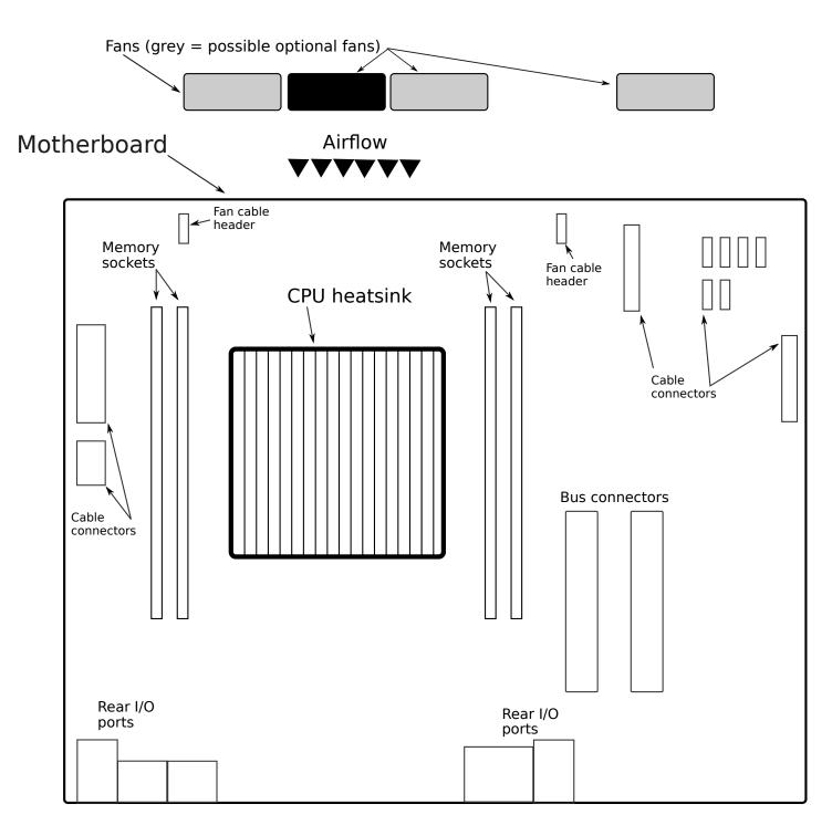
CPU heatsink fins, motherboards sockets of all types, cable connectors are all placed and situated to be parallel in length in order to optimize and smooth airflow.
