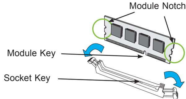
3. Press the SODIMM module straight down into the socket with both hands until it is securely seated in the socket. The side clips will automatically lock the module into place.
