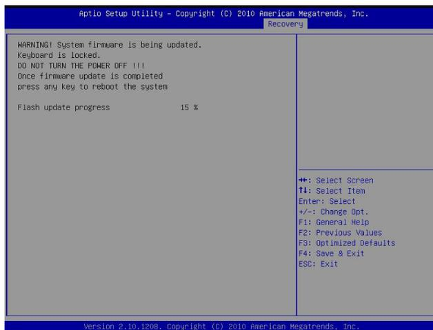
6. After the BIOS recovery process has completed, press any key to reboot the system.
