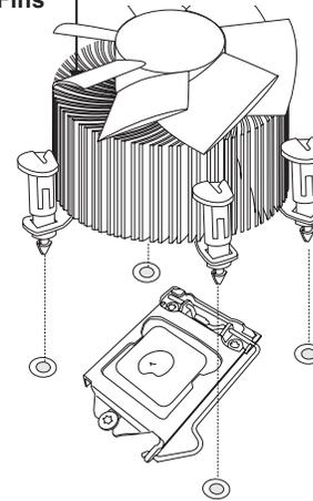
7. Align the four heatsink fasteners with the mounting holes on the motherboard. Gently push the pairs of diagonal fasteners (#1 & #2, and #3 & #4) into the mounting holes until you hear a click. Also, make sure to orient each fastener so that the narrow end of the groove is pointing outward.
