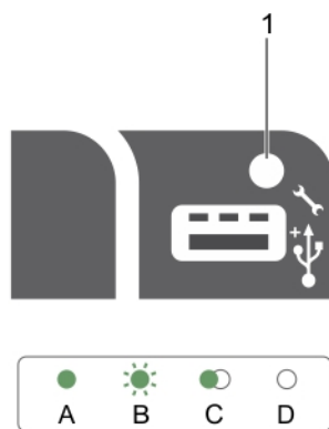
Figure 9. iDRAC Direct LED indicator
