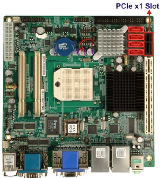
Figure 2-5: PCIe x1 Expansion Slot
