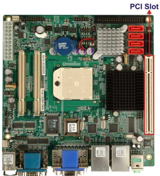
Figure 2-7: PCI Expansion Slot
