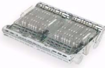
Figure 12. An optional memory mezzanine tray doubles memory capacity of the Sun Netra T5440 server.
