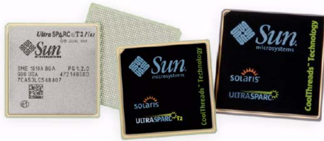
Figure 3. The UltraSPARC T2 Plus, UltraSPARC T2, and UltraSPARC T1 processors all take advantage of CoolThreads technology.
